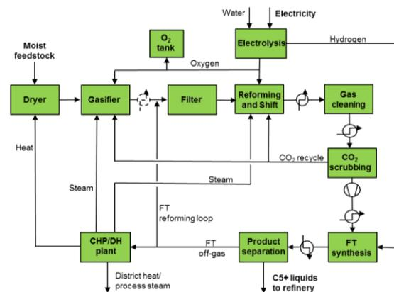
**Figure 3:** FLEXCHX process with electrolysis boosting and FT off-gas recycling.
