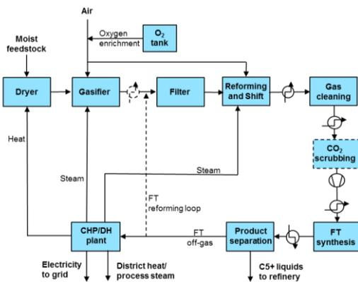
**Figure 2:** FLEXCHX process operated with biomass-alone during heating season.
